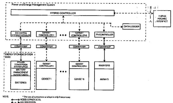
Figure 1: PEMS and Communication Diagram
